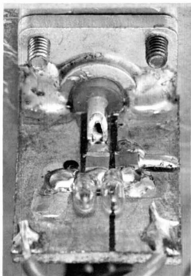
Construction of the rf sensor showing the two incandescent lamps and chip capacitors C1, C2. Components are mounted on a small section of double-clad PC board which is soldered to the rear flange of the BNC connector.
